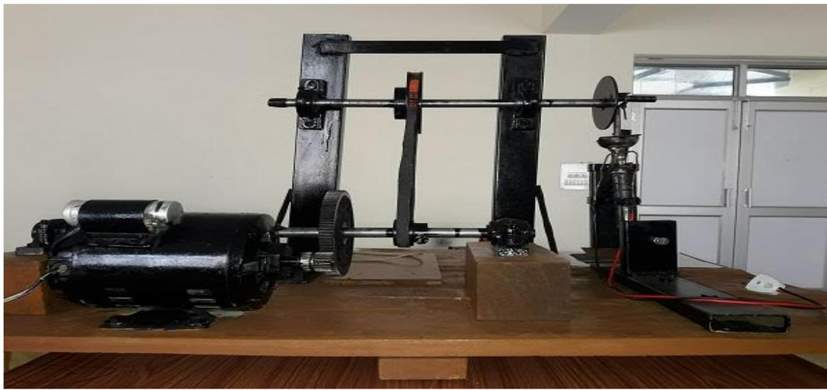
This machine consist power transmission system and SCOTCH YOKE MECHANISM. Power transmission system transfer power from motor to final shaft on which scotch yoke mechanism is installed, this mechanism convert rotatory motion into reciprocating motion. A punch is connected to scotch yoke mechanism which compresses the molten plastic material into the die through nozzle. After solidification desired product is obtained.
